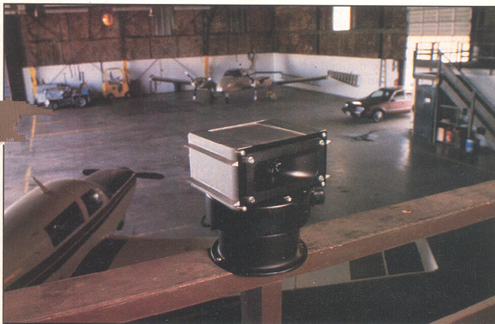
An ultrasonic device is being used in the hangars of Richland Aviation in Mansfield, Ohio, to keep the birds at bay.
